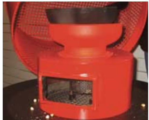
A working model of a pellet stove that can replace coal-fired ovens and stoves in for example China.
